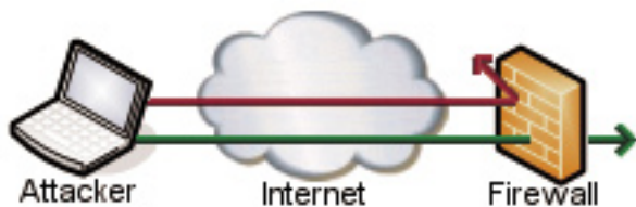
Figure 1: Attacks are blocked on closed ports, while open ports allow traffic through.
